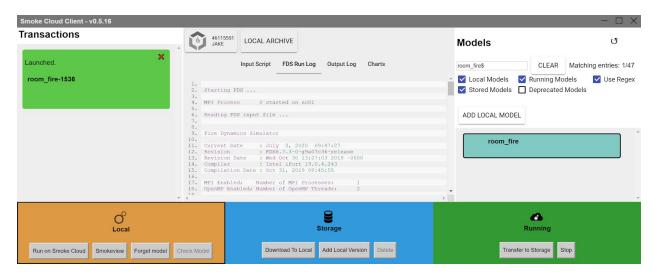
Stopping the model will stop the model, however far it is come, and transfer the results to storage. Pressing the transfer button will transfer a current snapshot of the simulation to storage for download, but will allow the simulation to continue running.
